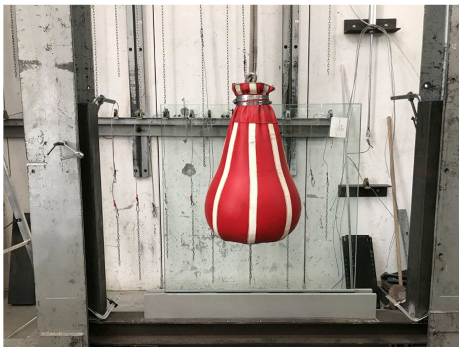
Photograph of the item after impact on the center of the glazing with dynamic load according to standard UNI 10807:1999
