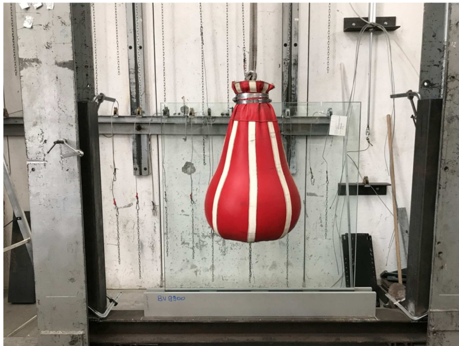
Photograph of the item after impact in the center of the glass
